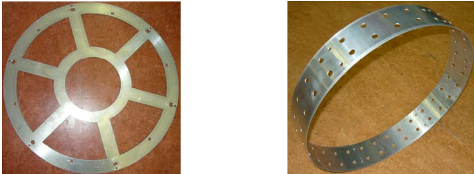
Figure 5.8: Stator housing and cover to protect against possible PM detachment.
