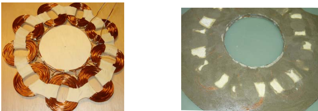
Figure 4.17: Manufacture of air cored stator: left photo shows arrangement of coils in a mould while right photo shows the completed stator.
