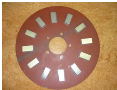
Figure 5.6: Photo of completed rotor disk. The hub connects the two rotor disk via the holes drilled on the disks and hub.
